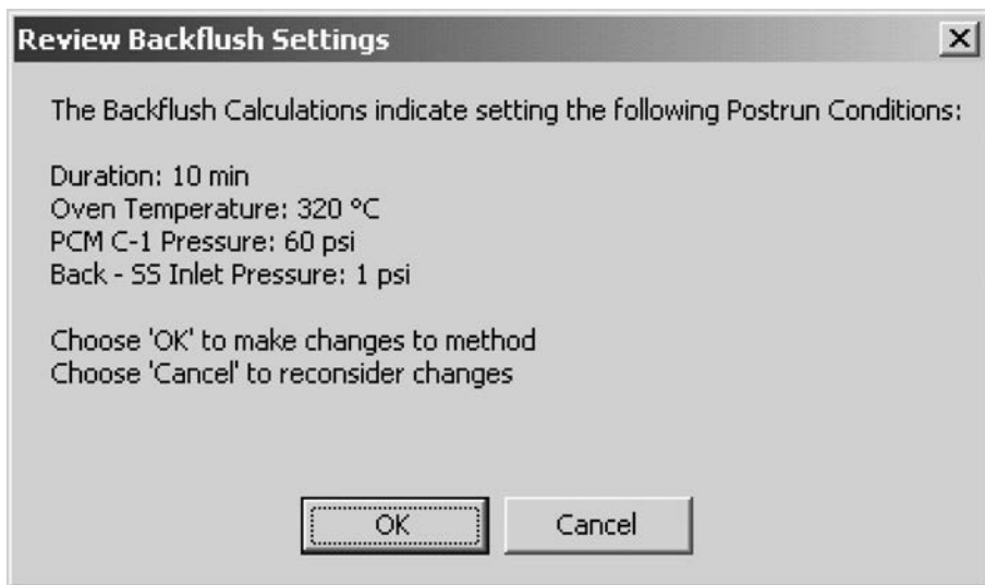
Figure 8. Post-run backflushing screen number 3.
