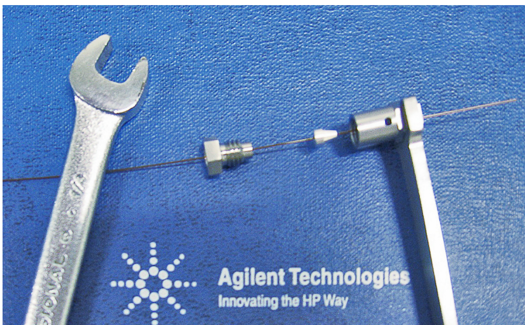
Figure 6 Thread the internal nut, ferrule, and ferrule pre-swaging tool
