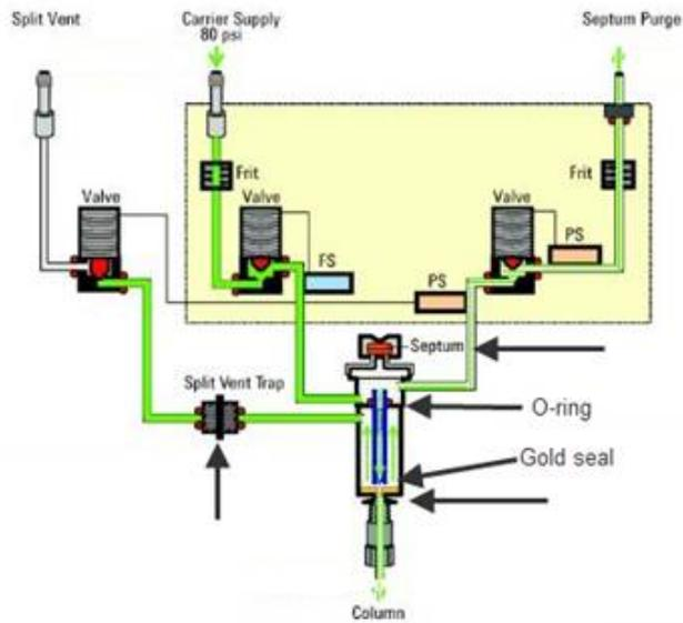
The leak check process checks for leaks in the column fitting, septum nut, weldment nut, split vent trap housing and gold seal fitting.
