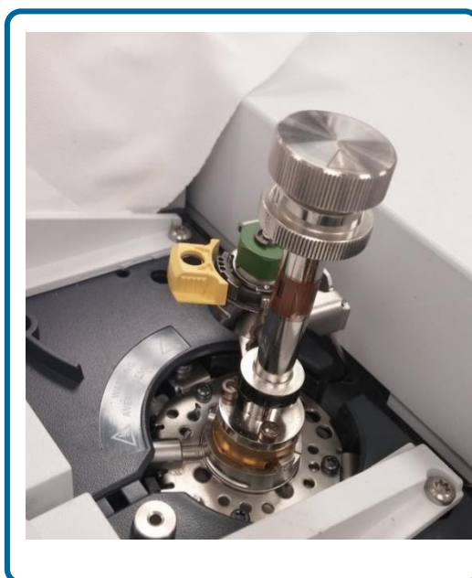
Figure 2: The TSP inserted into the GC Inlet
