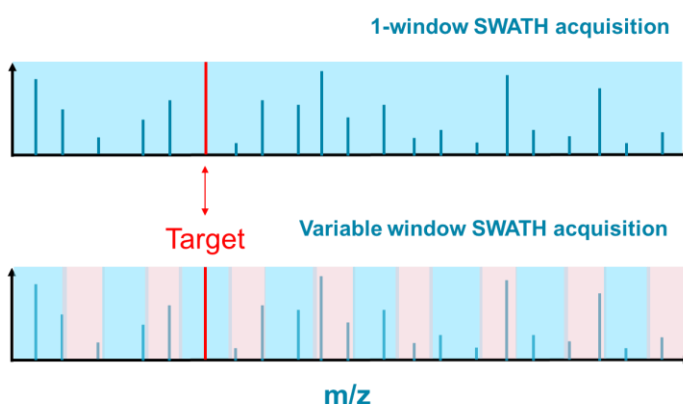
Figure 8: Impact of Number of Q1 Isolation Windows When Using SWATH Acquisition. One window SWATH Acquisition (top) uses 1 very large Q1 isolation window to select precursors for MS/MS, and therefore produces highly convoluted MS/MS spectra of everything eluting off the column at that point in time. When using multiple variable-sized windows during SWATH Acquisition (bottom), many fewer precursors are selected due to the much narrower isolation window, leading to MS/MS spectra that is much simpler and therefore easier to interpret.
