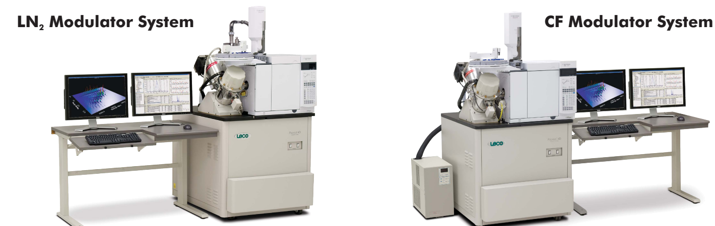
Figure 3. A LECO Pegasus® 4D utilizing the LN 2 modulator (left) and a LECO Pegasus 4D utilizing the CF Modulator (right). Note the absence of the liquid nitrogen dewar (to the left of the autosampler) on the CF Modulator system.
