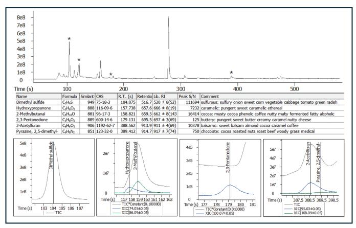
A chromatogram and peak table with representative analytes are shown for the non-target characterization of molasses with the Pegasus BTX. GC-TOFMS and the associated deconvolution algorithms can help you find non-target analytes at high S/N, low S/N, and when coeluting with other features in the sample, as shown with the highlighted examples. These uncovered features have interesting aroma characteristics and likely contribute to the complex aromas of molasses.
