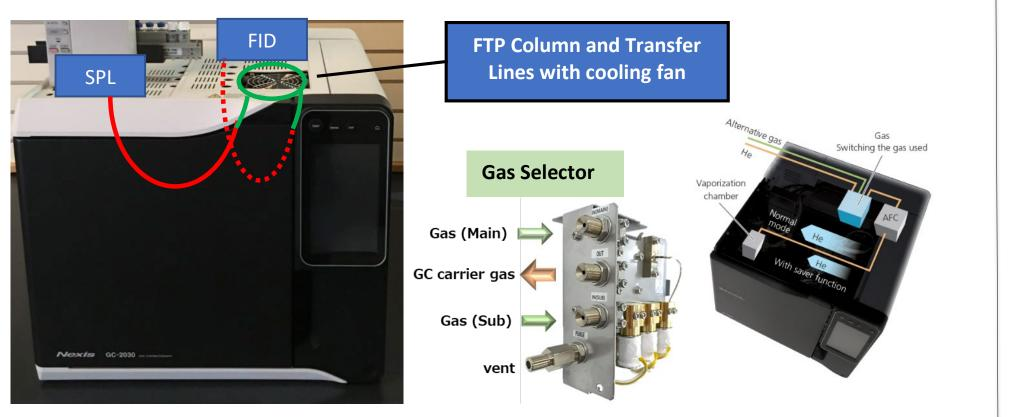
Figure 1: Ultrafast GC system with FTP column and gas selector.
