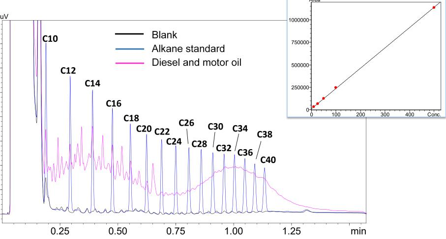
**Figure 2.** The Chromatograms of blank (dichloromethane), alkane standard (C10-C40) and a mix of diesel #2 and motor oil. He carrier gas was used. Inset shows an example calibration curve for motor oil with He carrier gas.
