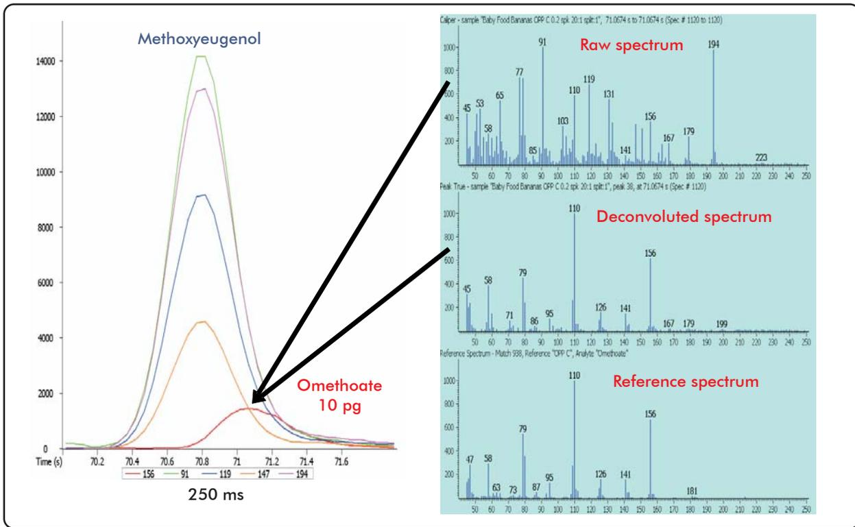
**Omethoate detected in baby food bananas and clearly identified despite coelution with methoxyeugenol.**
