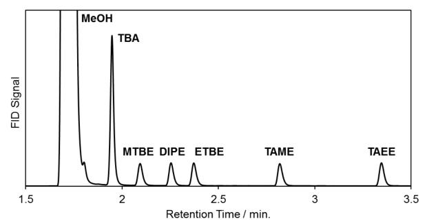
Figure 2. GC-Polyarc/FID chromatogram of oxygenates mixture.
