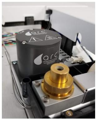
Figure 1. Polyarc Ultra on an Agilent 7890 GC.
