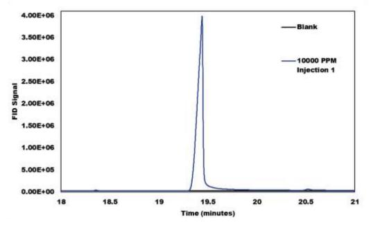
Figure 2. Polyarc/FID chromatogram of CBD isolate peak.
