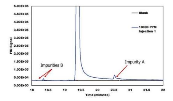
**Figure 3.** Polyarc/FID chromatogram of CBD peak with impurities A and B at minute 20.5 and 18.4 respectively.
