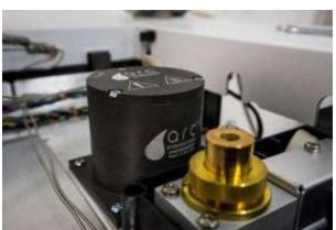
Figure 1. Polyarc microreactor on an Agilent 7890 GC.
