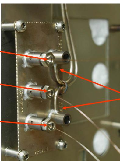
Pneumatic connections to the solenoid valve
