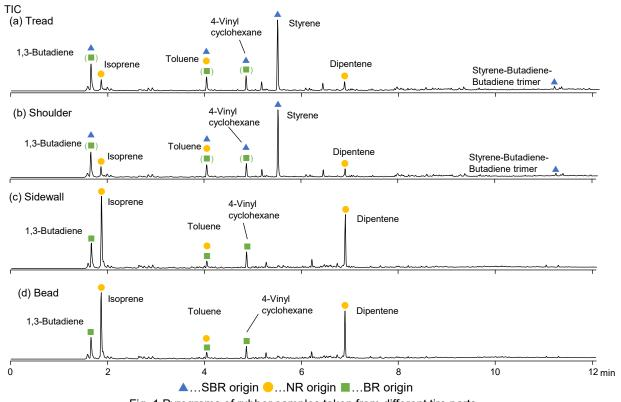
Fig. 1 Pyrograms of rubber samples taken from different tire parts
