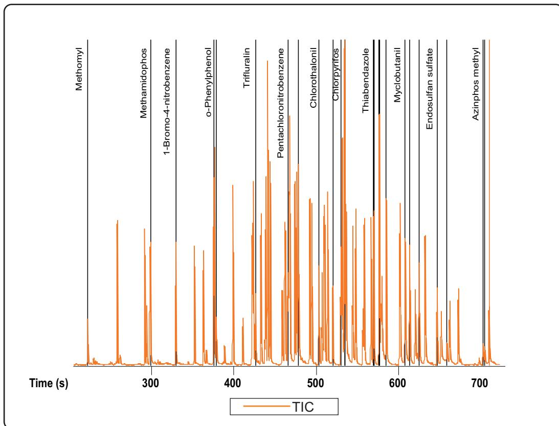
The total ion chromatogram shows the high point (1000 pg/µL) standard for the quantitative calibration range from 10 to 1000 pg/µL used to quantify pesticides in fruit and vegetables by GC-TOFMS analysis.
