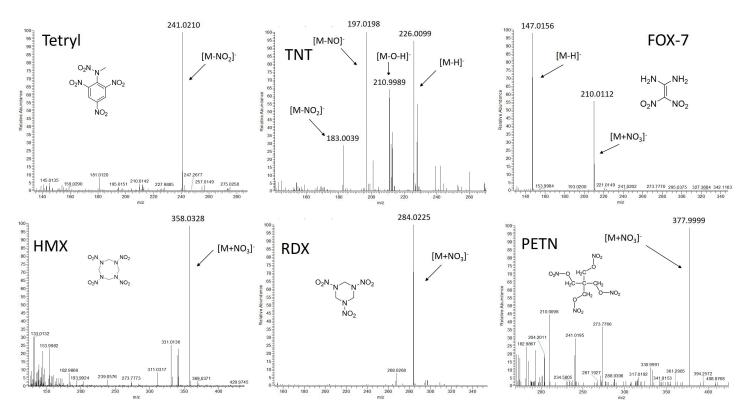
Figure 1 - Full MS spectra of investigated explosives (3 ng absolute) in negative mode, obtained on LTQ Orbitrap XL (Thermo Fisher).
