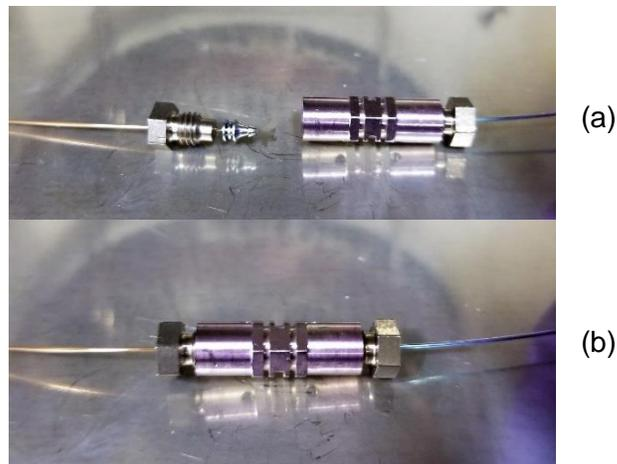
**Figure 9.** Inlet of the Polyarc® system connected to GC capillary column. (a) From left to right: column nut, capillary metal ferrule for GC column, zero-dead volume union. (b) Completed connection of components.
