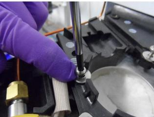
6. Prior to completing this step, you will need to replace the cover that was removed in Step #1 – The cover is removed in the pictures to show the important points of Step #6. Carefully insert the Polyarc into the inlet position opening, making sure that the Polyarc tubes are lined-up with the slot in the insulation. Avoid bending or kinking any of the tubes. When the Polyarc is properly positioned, the enclosure should not be touching any of the surrounding plastic.
