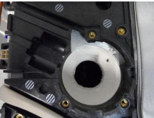
3. Place the provided disk of insulation into the opening. The Polyarc enclosure gets hot during use, conducting heat from the GC oven. Placing the insulation between the top of the oven and the bottom of the Polyarc enclosure will help reduce the amount of heat conduction, and the temperature of the micro-enclosure.
