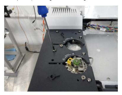
2. Remove back inlet position cover by removing 3 fasteners using a T20 driver, removing any insulation to uncover the hole that goes into the GC oven.
