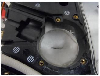
4. Place one of the supplied washers on each of the fasteners from the inlet cover that was removed in Step #2.
