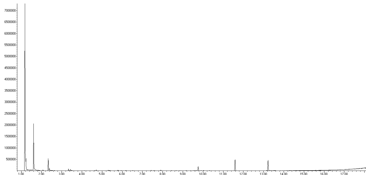
Figure 2: Dynamic Headspace Sampling Chromatogram of 5mL Yogurt Solution
