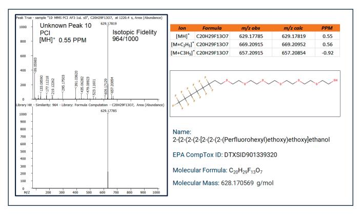
Figure 6. PCI Data and structural determination of unknown peak 10, using ChromaTOF° software with high-resolution accurate mass data for molecular adducts and subsequent search of the molecular formula with the EPA CompTox Chemicals Database.
