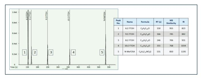
Figure 4. A zoomed-in section of the chromatogram section is highlighted in Figure 3A, and a table, showing 5 target PFAS species that were identified using standards and library data. Nomenclature used corresponds to the alkyl chain of the perfluorinated, and functional group sections of the compounds. For example, 6:2 FTOH represents a perfluorinated 6-carbon backbone tail, with an ethanol head.
