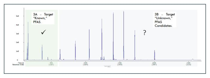
Figure. 3. Simultaneous target and non-target screening of a commercially available "anti-fog," spray. Sections of "known," PFAS targets (3A. highlighted in green) and "unknown," PFAS candidates (3B. highlighted in grey) are displayed.
