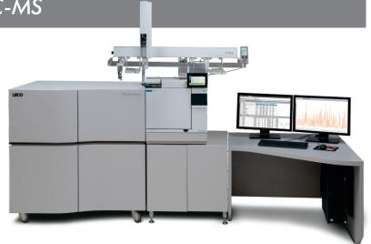
The new MMS has great mass accuracy and high resolution on pseudo-molecular ions, which complements the traditional Electron Ionization Source (HR-EI) to provide the comprehensive characterization of unknowns. By not touching the hardware, peaks stay aligned between the ionization modes. Each of the three modes is available for GC-MS and GCxGC-MS analyses on both the Pegasus® GC-HRT+ and Pegasus GC-HRT+ 4D.
