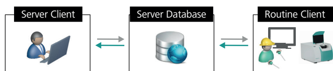
Figure 2. General setup of a client-server system for quality control. The setup consists of three elements: server client, routine client, and server database
