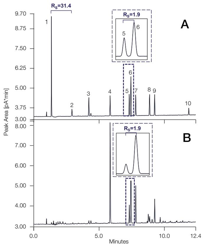
1=Methanol (A<sub>s</sub>=1.2), 2=Methyl-*tert*-butylether (MTBE, A<sub>s</sub>=1.0), 3=Benzene (A<sub>s</sub>=1.0), 4=Toluene (A<sub>s</sub>=1.0), 5=Ethylbenzene (A<sub>s</sub>=1.0), 6=*m,p*-xylene (A<sub>s</sub>=1.0), 7=*o*-xylene (A<sub>s</sub>=1.0), 8=2,3,5-trimethylbenzene (A<sub>s</sub>=1.0), 9=1,2,4-trimethylbenzene (A<sub>s</sub>=1.0), 10=Naphthalene (A<sub>s</sub>=1.0)
