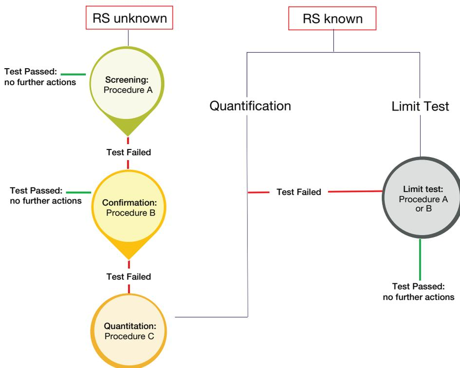
Figure 3. Simplified diagram of the analytical workflow used for residual solvent assessment
