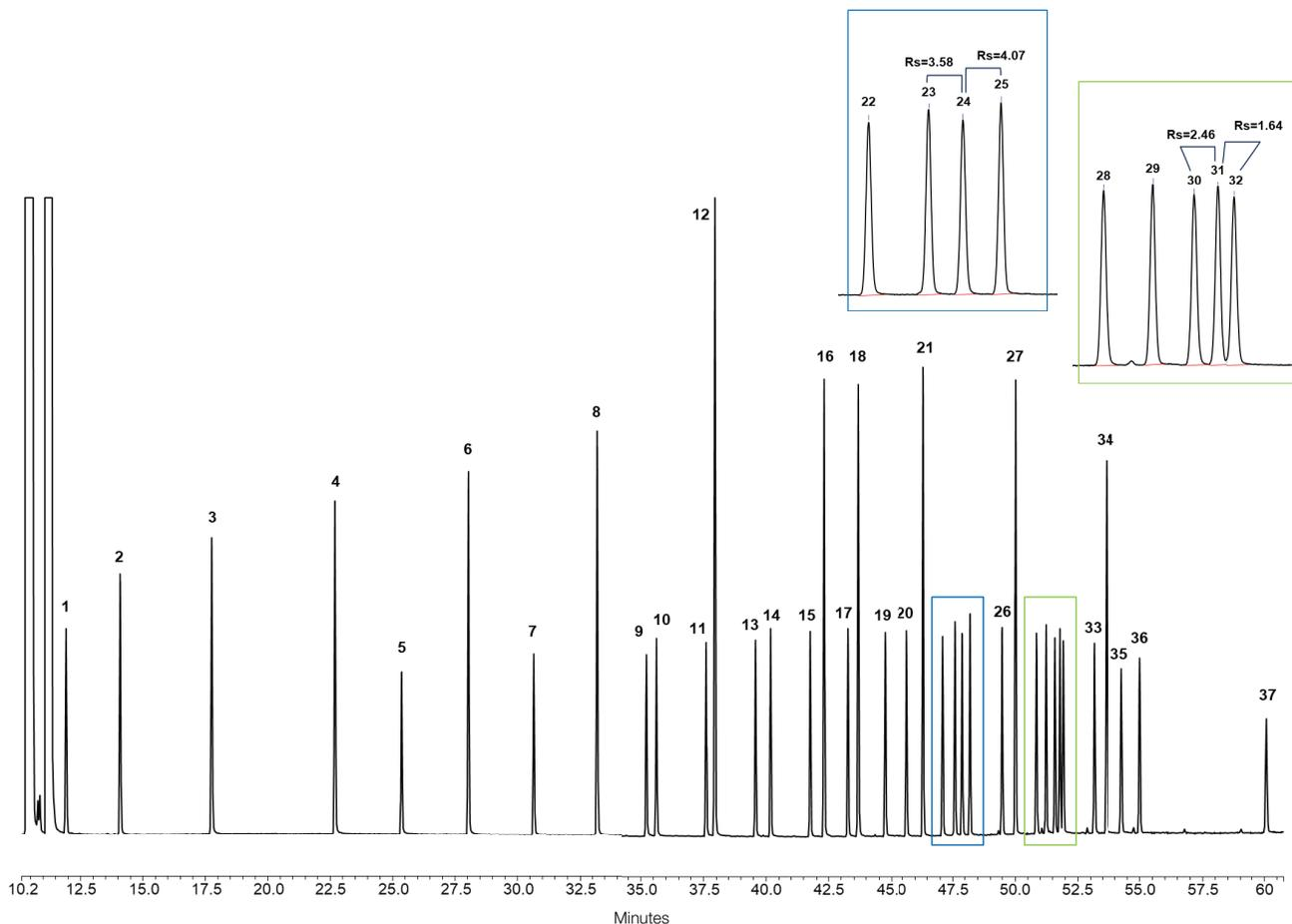
Figure 6. Chromatographic separation of a solvent standard of the Food Industry FAMES mix (37 components) at 50 ppm ( $\mu\text{g/mL}$ ) on column using the TRACE 1610 Gas Chromatograph and a Restek Rt-2560 column.
