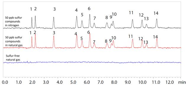
Figure 4: Stacked chromatograms showing the SCD-2030 response for a 50 ppb mix of sulfur compounds in nitrogen (black), in natural gas (red), and a blank, sulfur-free natural gas standard (blue). Note that the baselines have been shifted for comparative purposes.
