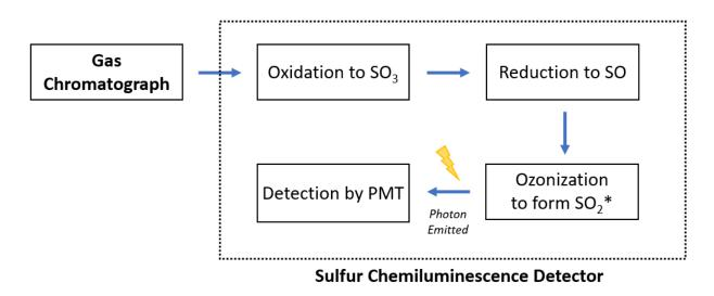
Figure 1: A simplified schematic of the operation of a sulfur chemiluminescence detector.
