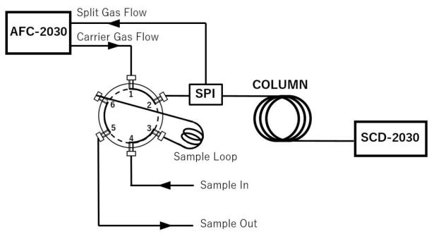
Figure 2: Schematic of instrument configuration.
