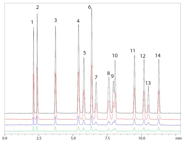
**Figure 3**: Stacked chromatograms of the calibration curve standards. Green = 50 ppb sulfur (v/v), Blue = 100 ppb, Red = 500 ppb, and Black = 1000 ppb. Note that the baselines have been shifted for comparative purposes.
