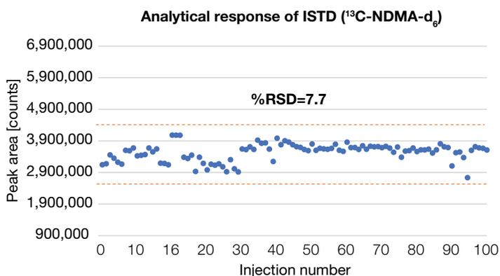
Figure 3. ISTD (<sup>13</sup>C-NDMA-d<sub>6</sub>) peak area % RSD obtained analyzing extracts (n=100) over a period of several weeks
