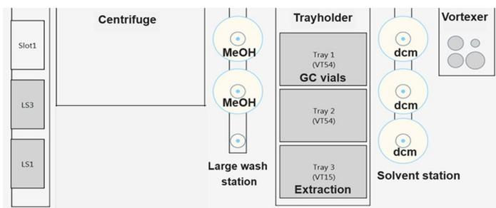
**Figure 1. TriPlus RSH SMART autosampler configuration for automated extraction of nitrosamines from drug substance**
