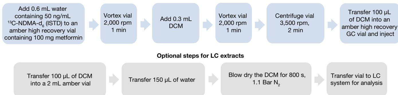
**Figure 2. Workflow showing the sample extraction procedure for GC and LC (optional)**
