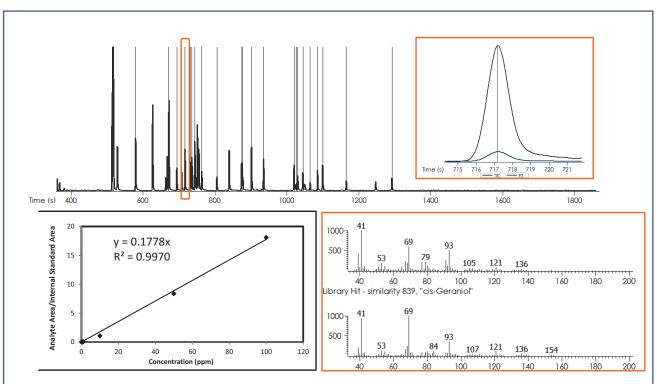
Figure 1. GC-TOFMS data were collected for an allergen standard, containing 24 of the regulated analytes. Allergens are indicated in the standard with vertical line peak markers, and geraniol is shown as a representative example. The peak profile, mass spectral information, and calibration data are compiled. Calibration equations for all analytes were determined with automated data processing, and can also be applied to subsequent unknown samples in an automated way.
