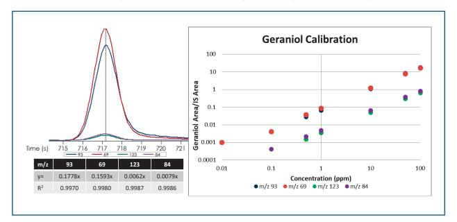
Figure 2. Geraniol is chromatographically isolated in the allergen standard and several m/z are unique and appropriate for determining calibration equations. m/z 93, 69, 123, and 84 are all free from interferences and provide reliable calibration information. SIM methods often suggest m/z 93, 69, and 123 for this analyte.
