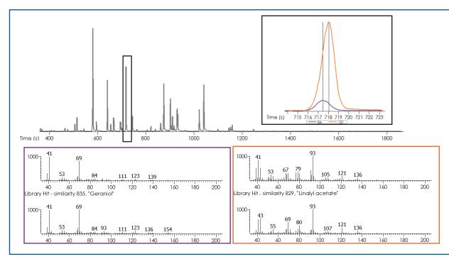
Figure 3. Geraniol, a target allergen, coelutes with a matrix analyte, tentatively identified as linalyl acetate. ChromaTOF's deconvolution capabilities mathematically separates this coelution and provides pure spectra and pure peak profiles for each analyte. There are several shared m/z between these analytes.
