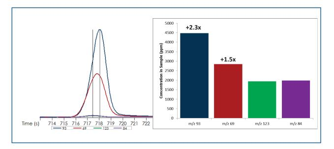
Figure 4. The target allergen and the coelution share multiple m/z, including m/z 93 and 69 that are recommended SIM masses. If quantification is done with these m/z, the reported concentration is skewed by the contribution of the matrix interference. m/z 123 and 84 have less interference from the coelution and provide more reliable quantification information.
