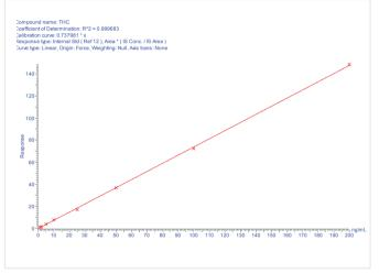
Figure 6. Typical Calibration line of THC at 1–200 ng/mL on ISOLUTE® SLE+ 1 mL sample volume columns
