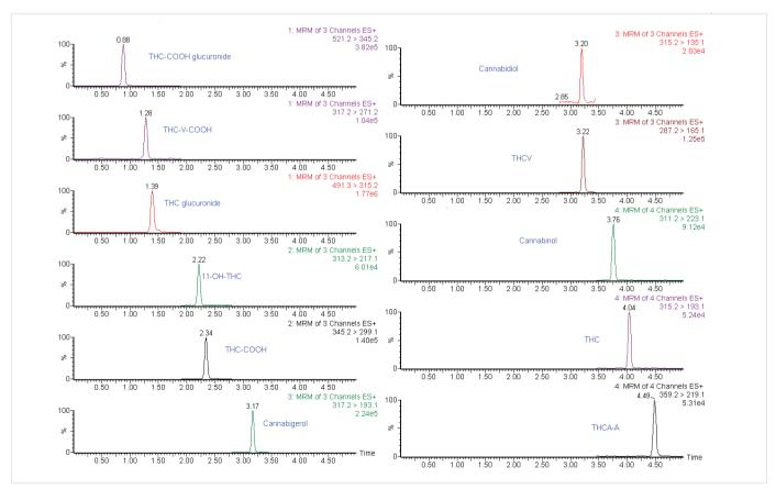
Figure 3. Typical MRM chromatogram of THC and metabolites at 5 ng extracted using the method described for ISOLUTE SLE+ 400 µL sample volume columns.
