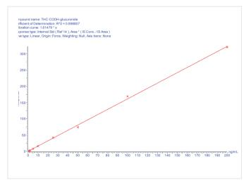
Figure 7. Typical Calibration line of THC-COOH glucuronide at 1-200 ng/ mL on ISOLUTE  $^{\otimes}$  SLE+ 1 mL sample volume columns
