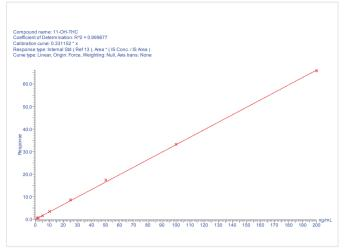
Figure 4. Typical Calibration line of 11-OH-THC at 1-200 ng/mL on ISOLUTE<sup>®</sup> SLE+ 1 mL sample volume columns
