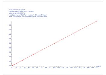
Figure 5. Typical Calibration line of THC-COOH at 1–200 ng/mL on ISOLUTE $^{\otimes}$  SLE+ 1 mL sample volume columns
