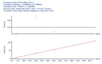
**Figure 8.** Chromsystems Calibrated Serum Curve for 25-OH vitamin D3 constructed from 0-58 ng/mL.
