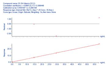
**Figure 7.** Chromsystems Calibrated Serum Curve for 25-OH vitamin D2 constructed from 4-69 ng/mL.
