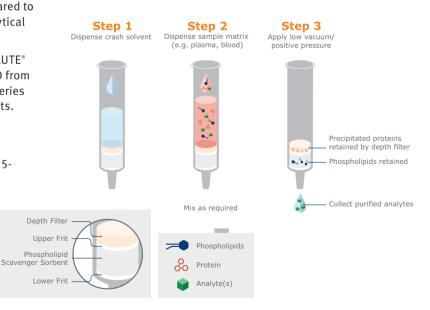
Figure 2. Typical ISOLUTE® PLD+ procedure
