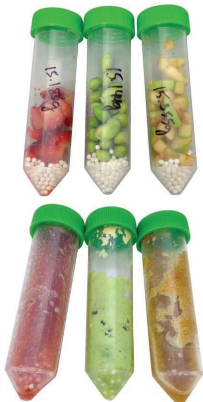
**Figure 1.** Produce Samples Pre and Post Homogenization. 15 g samples of strawberry, soybeans, and apples were homogenized on the Biotage® Lysera with 15 g of ceramic beads in 30 seconds.
