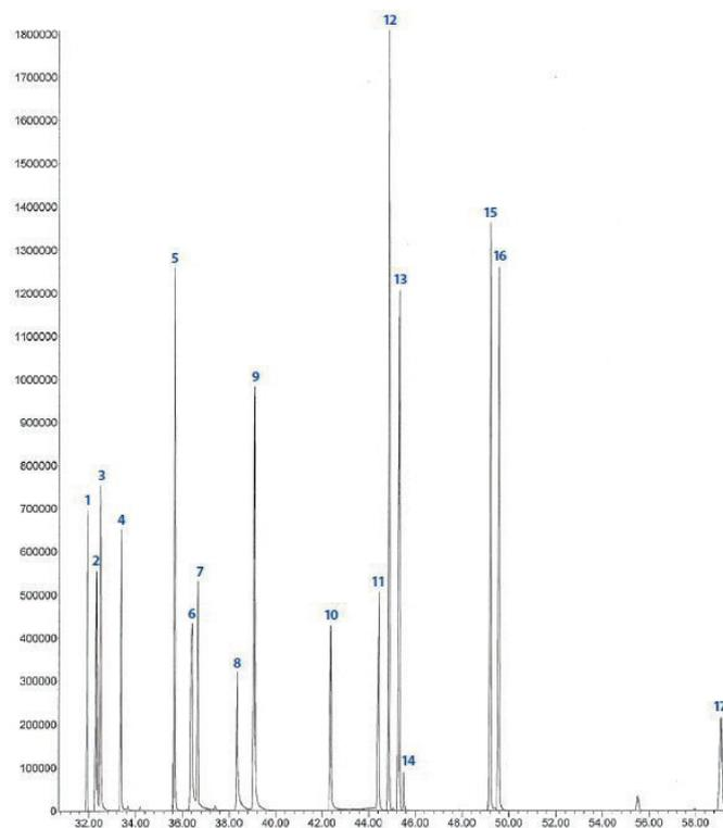
**Figure 2.** GC-MS Total Ion Chromatogram – 100 ppb Spiked Strawberry Sample. TIC displays the elution profile of the 17 pesticide standards extraction from the 100 ppb spiked strawberry sample post QuEChERS extraction.
