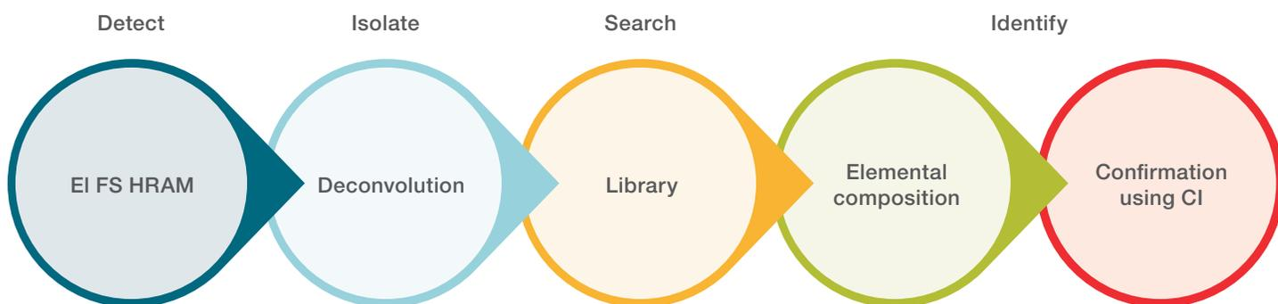
**Figure 1. Workflow for non-targeted screening of vial septa.** Full scan data were acquired using EI full scan HRAM; spectral deconvolution with library search for putative compound identification; and confirmation using chemical ionization (CI) data, for added specificity and selectivity.
