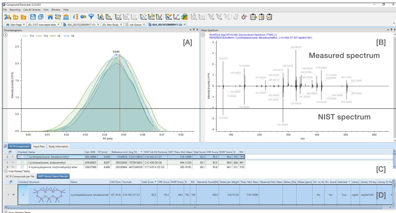
Figure 3. Compound Discoverer software deconvolution results for a range of the tested silicon / PTFE septa, for the compound eluting at RT= 9.55 min and putatively identified as tetradecamethyl-cycloheptasiloxane. [A] XIC for tetradecamethyl-cycloheptasiloxane; [B] Measured vs NIST20 library EI spectrum for tetradecamethyl-cycloheptasiloxane; [C] Result table with deconvoluted compound; [D] Library search results against NIST20.
