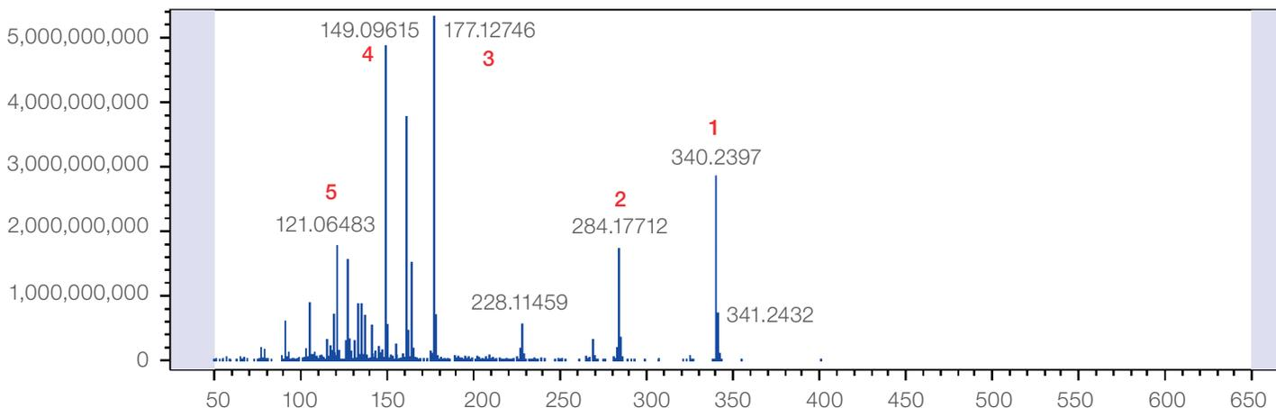
Figure 6. Mass Frontier software generated proposed structures for the ions generated in the mass spectra for the peak at 19.63 min in the natural rubber / TEF sample, against the top match of phenol, 2,2'-methylenebis[6-(1,1-dimethylethyl)-4-methyl-
