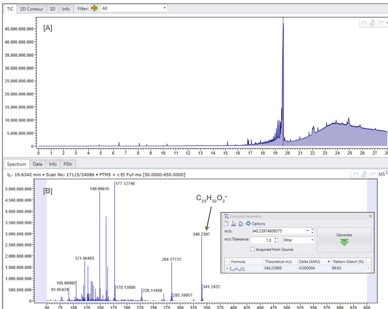
Figure 4. Mass Frontier structural elucidation software results used to aid identification of the elemental composition results for the peak at 19.63 min in the natural rubber / TEF septa sample. [A] TIC; [B] Mass spectra for the peak at 19.63 min, with Formula Generator results for the parent ion at  $m/z$  340.2397.
