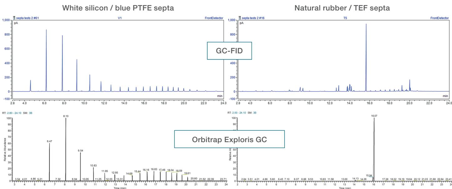
**Figure 2. GC-MS TICs for EI full scan data (bottom) and GC-FID data (top), obtained for septa sample (white silicon / blue PTFE) and septa sample (natural rubber / TEF)**
