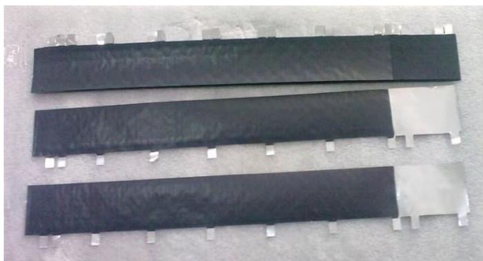
Figure 1. Li-ion battery electrodes
