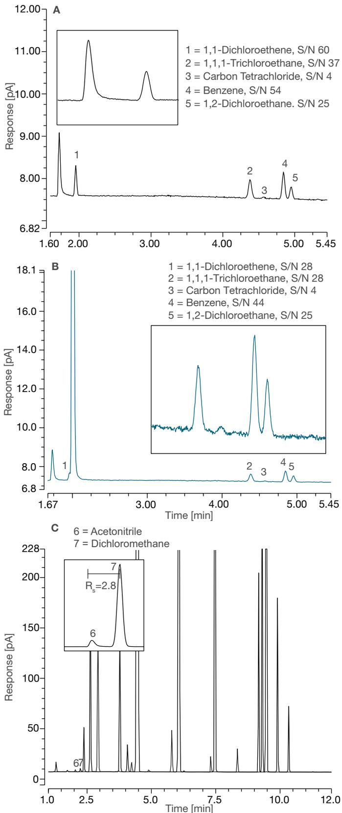
Figure 4. USP <467> system suitability requirements were met for both Class 1 and Class 2 residual solvents with: peak-to-peak S/N for 1,1,1-trichloroethane in Class 1 standard solution >5:1 (A); peak-to-peak S/N of each peak in Class 1 system suitability >3 (B); and resolution between acetonitrile and dichloromethane in Class 2 standard solution >1.0 (C)
