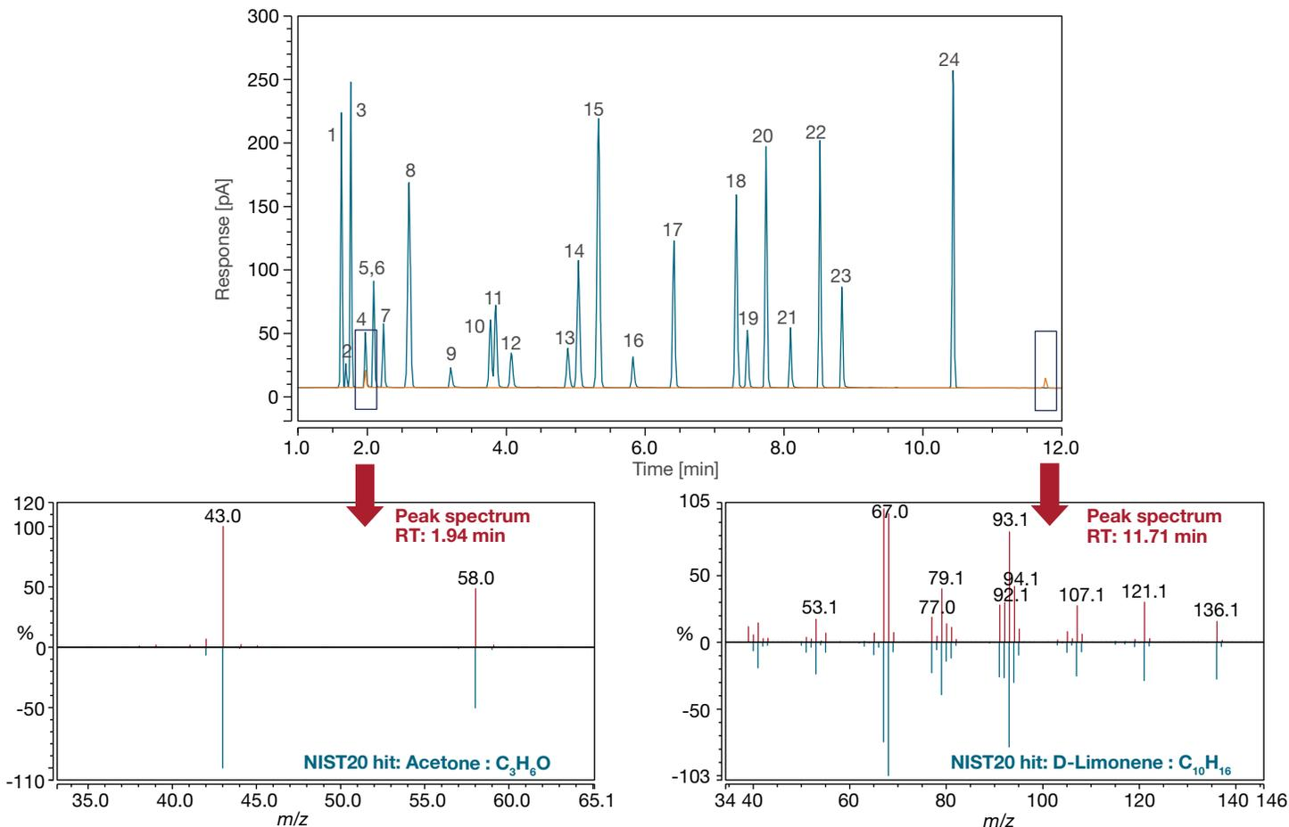
Figure 2. Comparison between Class 3 limit test solution (blue) and acetylsalicylic acid solution (orange). Residual acetone was found to be below the limit threshold of 5,000  $\mu\text{g/g}$  (or 50 mg/day). D-Limonene was also identified in the sample, in agreement with the ingredients declared by the manufacturer.
