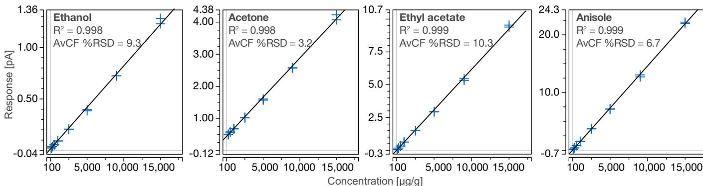
Figure 3. Examples of calibration curves obtained by injecting a seven-point matrix-matched calibration curve ranging from 100  $\mu\text{g/g}$  to 15,000  $\mu\text{g/g}$  (corresponding to 1 mg/day to 150 mg/day). Each calibration point was prepared in duplicate.
