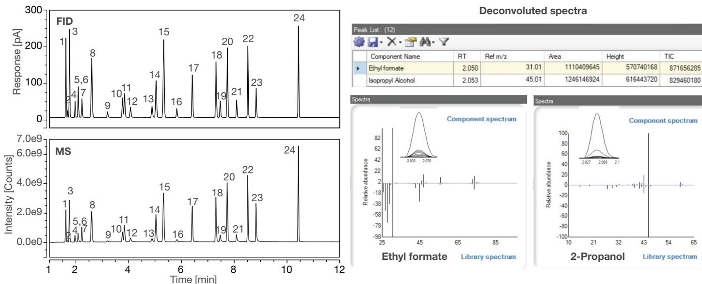
1=Pentane, 2=Ethanol, 3=Ethyl ether, 4=Acetone, 5=Ethyl formate, 6=2-Propanol, 7=Methyl acetate, 8=tert-Butylmethyl ether, 9=1-Propanol, 10=2-Butanone, 11=Ethyl acetate, 12=2-Butanol, 13=Isobutanol, 14=Isopropyl acetate, 15=Heptane, 16=1-Butanol, 17=n-Propyl acetate, 18=Methylisobutylketone, 19=3-Methyl-1-butanol, 20=Isobutyl acetate, 21=1-Pentanol, 22=Butyl acetate, 23=N,N-Dimethylformamide, 24=Anisole
