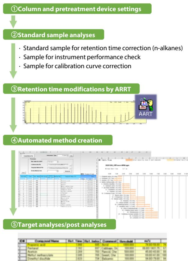
Fig. 1 Analysis Flow with GC/MS Off-Flavor Analyzer
