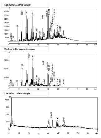
Fig. 1 Chromatograms of high, medium, and low sulfur content samples analyzed with the analytical column setup
