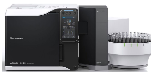
Fig. 3 Nexis™ GC-2030 + HS-20 NX (Loop Model)
