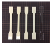
Fig. 1 Appearance of Specimens From left, PC : ABS = 0 : 100, 25 : 75, 50 : 50, 75 : 25, 100 : 0
