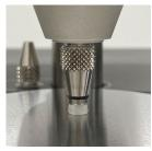
Fig. 3 Transparent Bead Pressed against the ATR Prism
