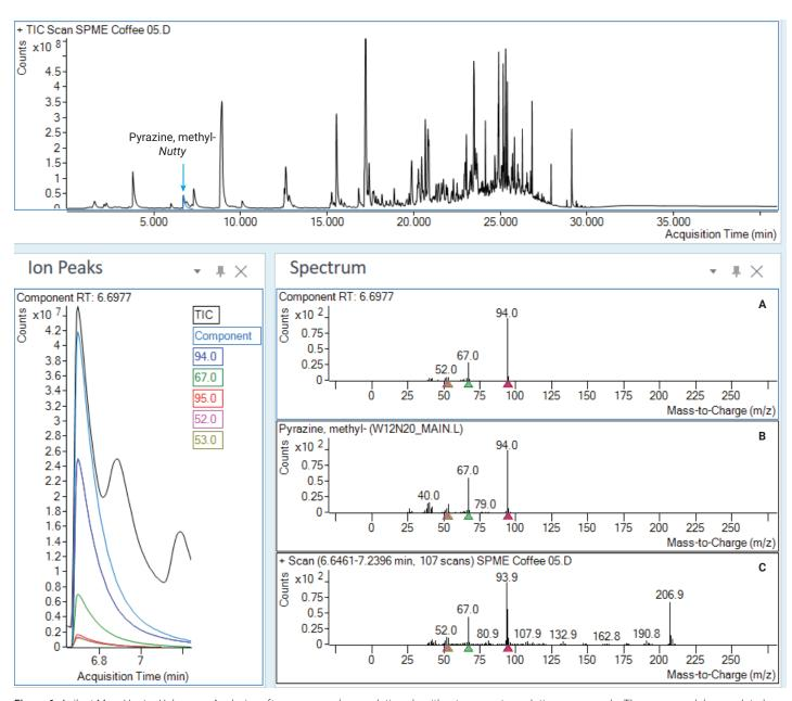
Figure 6. Agilent MassHunter Unknowns Analysis software uses a deconvolution algorithm to separate coeluting compounds. The compound deconvoluted spectrum (A), library spectrum (B), and raw spectrum (C) are displayed.
