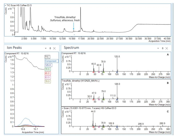
Figure 7. Agilent MassHunter Unknowns Analysis software uses a deconvolution algorithm to separate coeluting compounds. The compound deconvoluted spectrum (A), library spectrum (B), and raw spectrum (C) are displayed.
