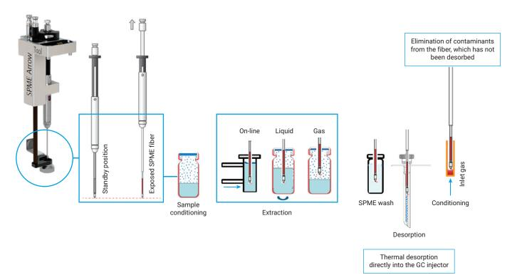
Figure 2. Schematic of SPME/SPME Arrow.
