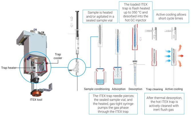
Figure 1. Schematic of dynamic headspace ITEX.
