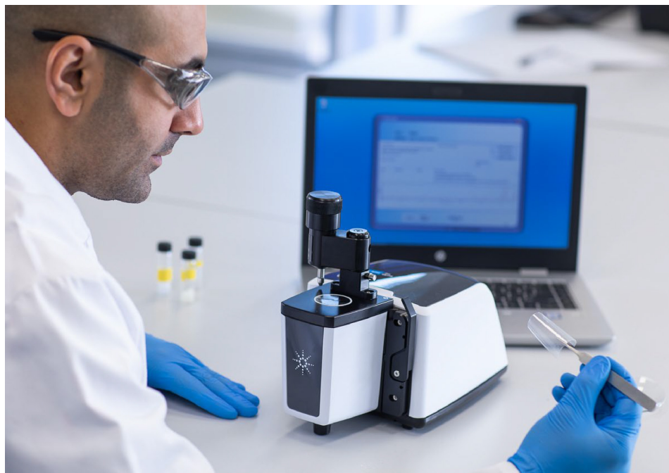
Figure 5. Agilent Cary 630 FTIR spectrometer coupled with a diamond ATR module.
