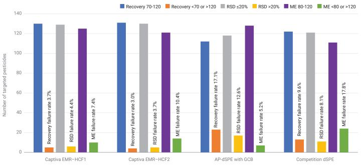
Figure 4. Targeted pesticides statistical comparison for recovery, RSD, and matrix effect (ME) in spring mix samples prepared by Agilent Bond Elut QuECHERS AOAC extraction followed with different cleanup methods. Spiking level at 10 ng/g in spring mix.
