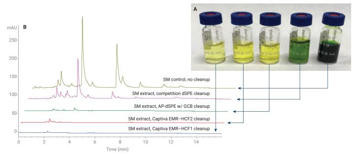
Figure 3. Spring mix (SM) matrix sample pigment removal efficiency demonstration. (A) Extracted samples color comparison. (B) LC-UV ( $\lambda$  = 450 nm) stacked chromatograms for extracted spring mix samples.
