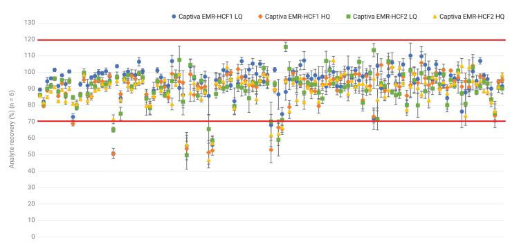
Figure 6. Target accuracy and precision results in spring mix. Two levels of pre-spiking include 10 ng/g for LQ and 100 ng/g for HQ. Samples were prepared using Agilent Bond Elut QuEChERS AOAC extraction kit followed by Agilent Captiva EMR-HCF1 and Captiva EMR-HCF2 cleanup, respectively.
