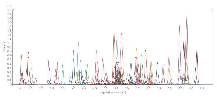
Figure 1. LC/MS/MS MRM chromatogram for extracted spring mix sample fortified with 100 ng/g of 130 targeted pesticides. The sample was prepared using the Agilent Bond Elut QuEChERS AOAC extraction kit, followed by Agilent Captiva EMR-HCF1 cleanup.
