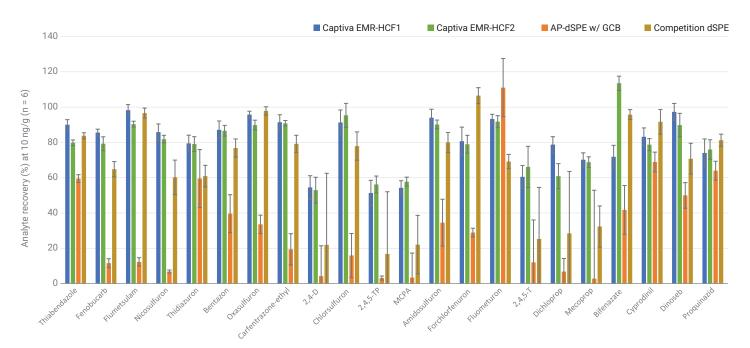
Figure 5. Sensitive target recovery results comparison for samples prepared using different cleanup methods.
