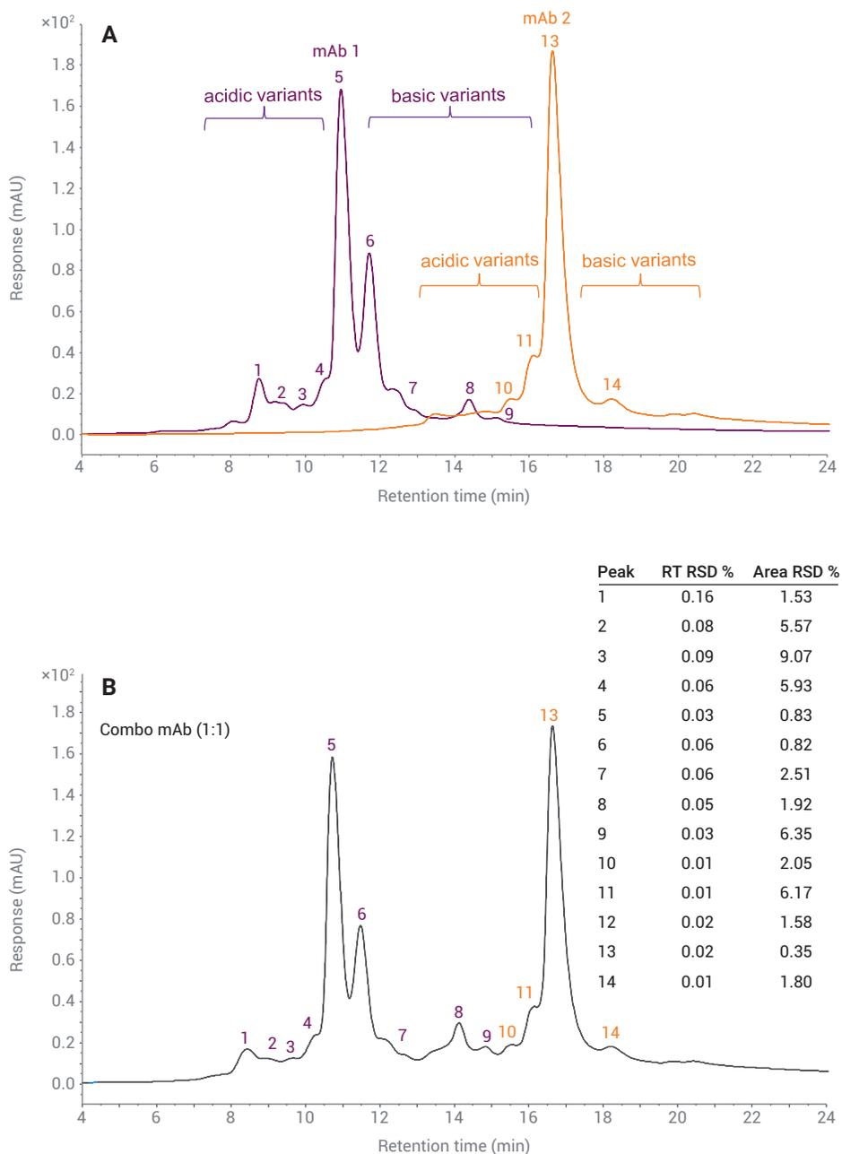
**Figure 1.** Cation-exchange chromatography profiles of mAb 1 and mAb 2 antibodies, individually formulated (A) and after coformulation (1:1) (B) on the Agilent Bio Mab, NP5, 2.1 × 250 mm, PEEK.
