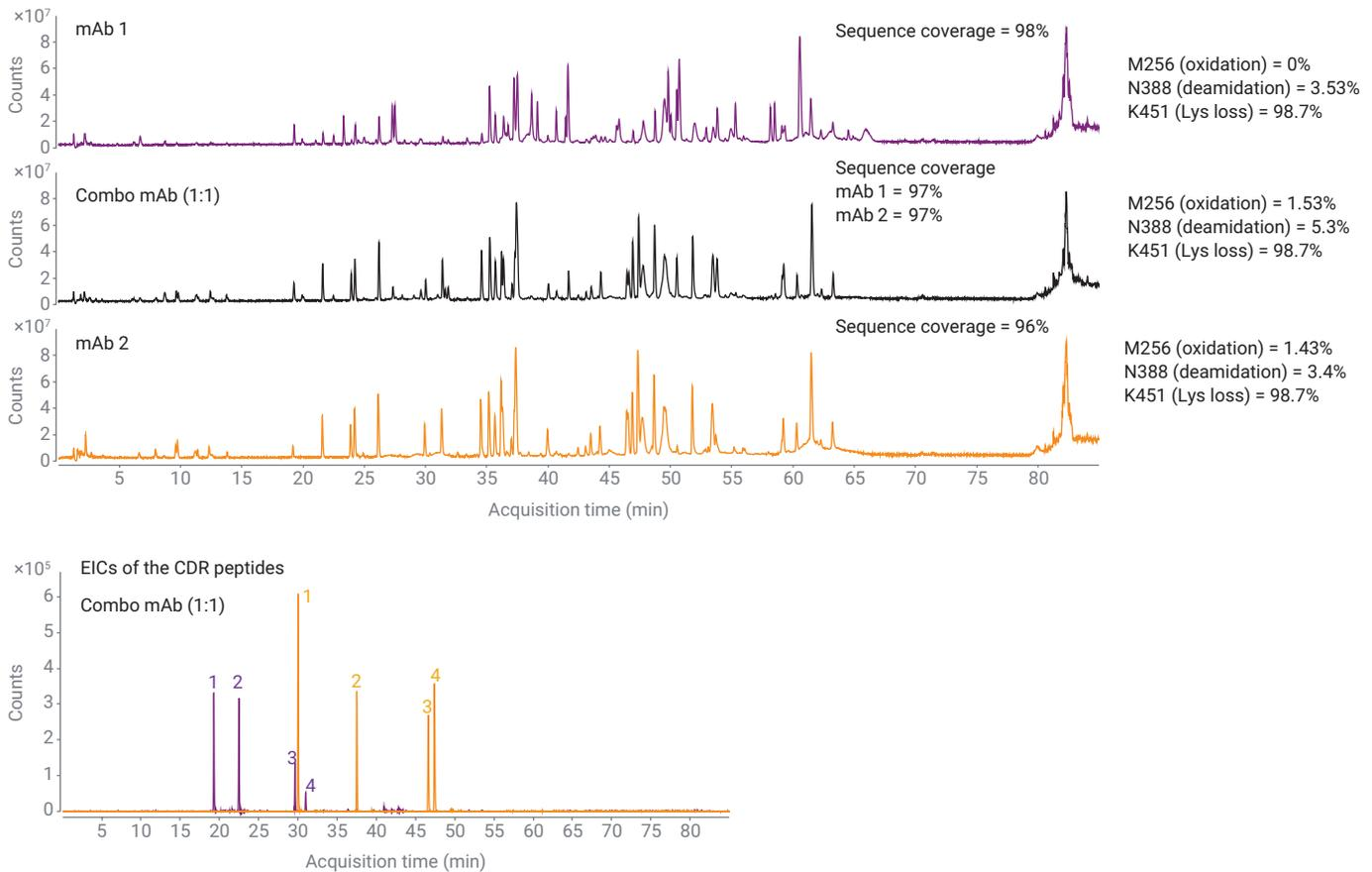
**Figure 3.** LC/MS separation of tryptic digest with an Agilent AdvanceBio peptide mapping column. Total ion chromatogram (TIC) of mAb 1, mAb 2, and the 1:1 coformulated mAb mixture.
