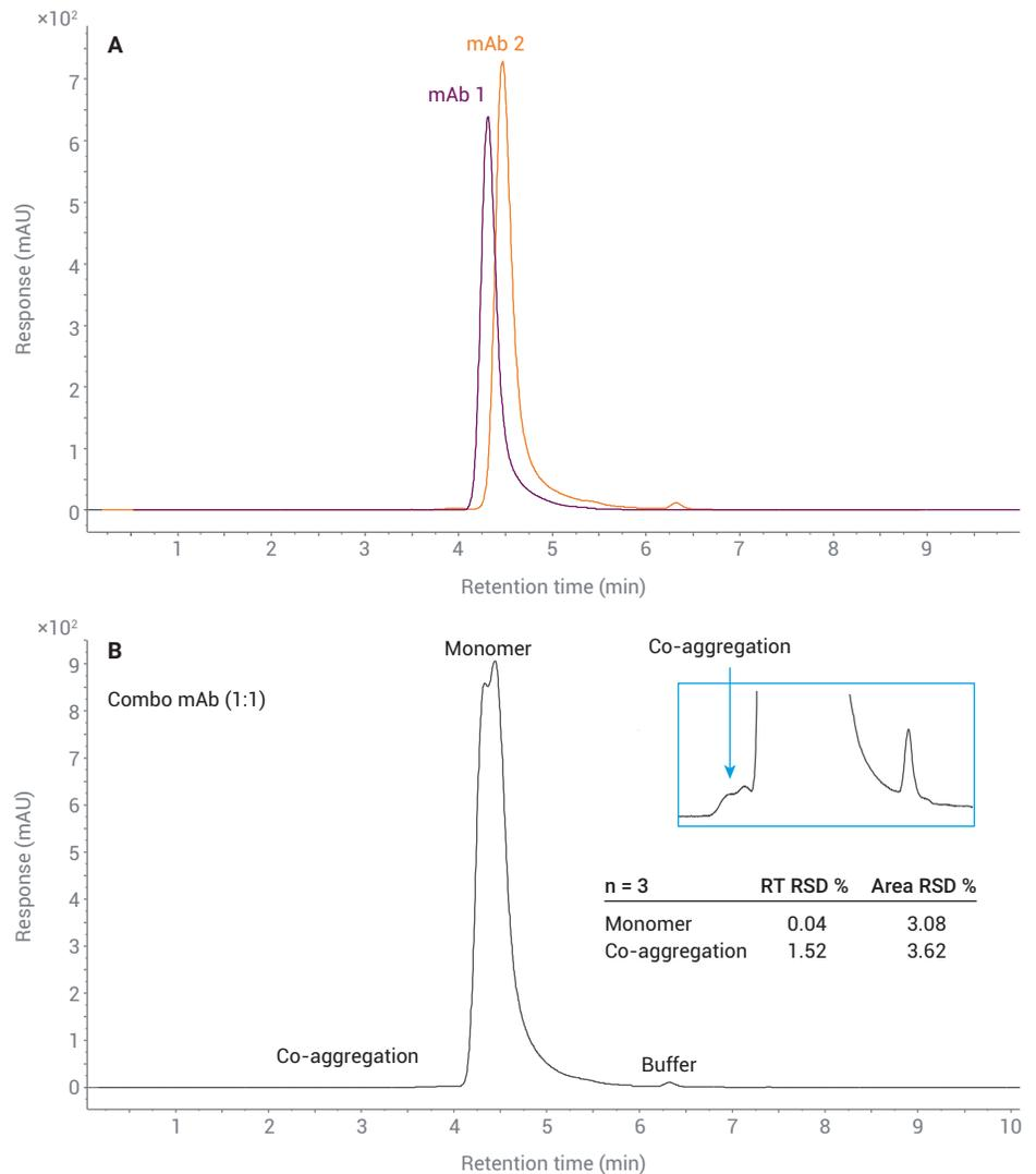
**Figure 2.** Size exclusion chromatography profiles of mAb 1 and mAb 2 antibodies, individually formulated (top, A) and after coformulation (1:1) (bottom, B) on the AdvanceBio SEC 300Å, 7.8 × 300 mm, 2.7 μm.
