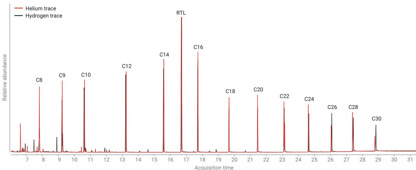
**Figure 1.** Comparison of the FAMES calibration standards using helium (red) and hydrogen (black).
