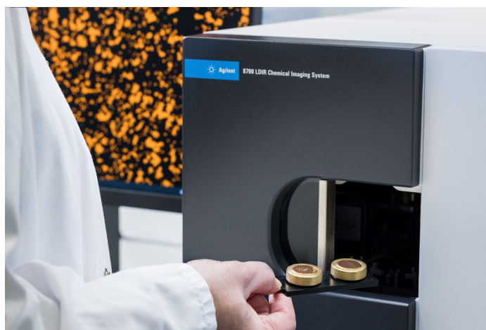
Figure 1. The Agilent 8700 LDIR chemical imaging system allows the high-speed routine analysis of microplastics, including reporting the number of particles present in a sample, size of particles, and chemical composition (identity) of particles.
