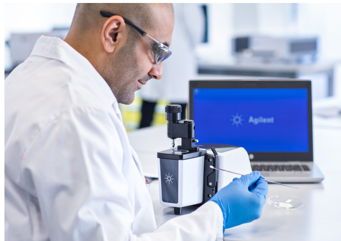
Figure 2. The Agilent Cary 630 FTIR spectrometer coupled with a diamond ATR module and controlled using Agilent MicroLab software is widely used for the accurate and reliable ID of materials.
