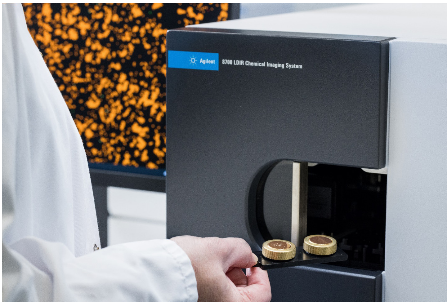
Figure 1. The Agilent 8700 LDIR Chemical Imaging System allows the high-speed routine analysis of microplastics, including the number of particles present in the sample, their size, and their chemical composition.
