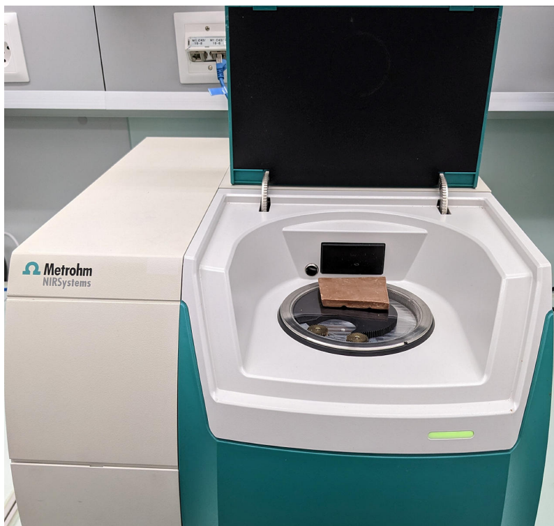
Figure 1. Metrohm NIRS DS2500 Solid Analyzer with a chocolate bar covering the sample window.
