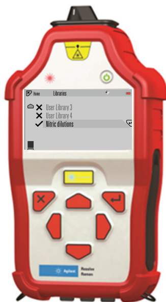
Figure 3. Agilent Resolve handheld Raman analyzer screenshots showing the details of the newly created "Nitric dilutions" library.
