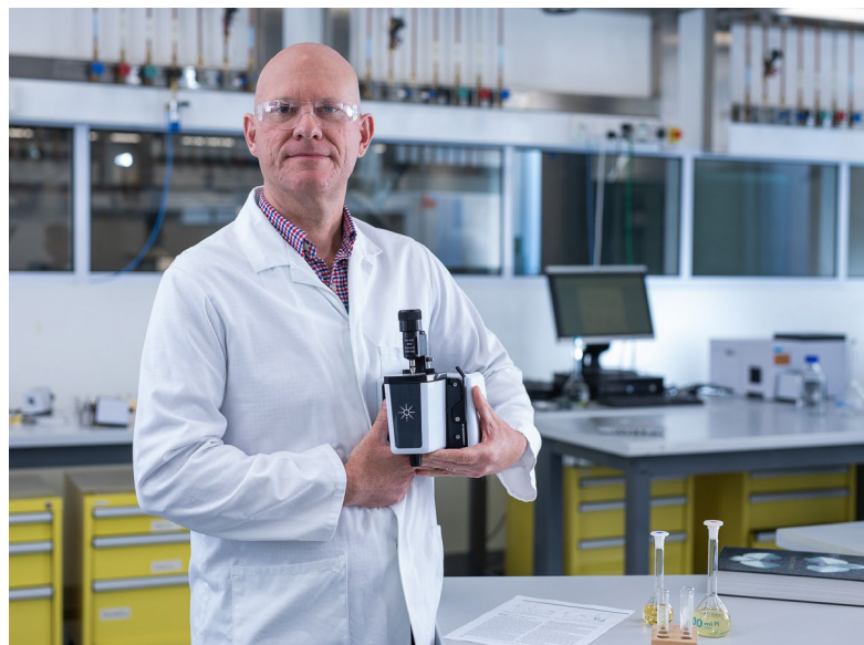
Figure 2. Agilent Cary 630 FTIR spectrometer with Diamond Attenuated Total Reflection sampling module attached.
