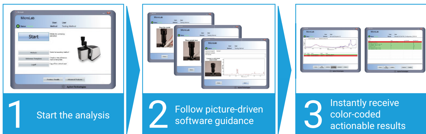
Figure 3. Agilent MicroLab software automatically recognizes the attached sampling module and applies the correct parameters. The software navigates the user, step-by-step, through the analytical workflow using instructive pictures. Color-coded results, directly reported after data acquisition, make data review quick and intuitive.
