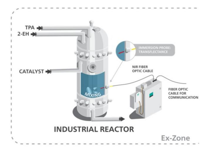
Figure 3. Stylization of suggested placement for near-infrared (NIR) probe in an industrial DOTP reactor.
