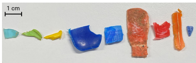
Figure 2. Plastic debris collected from a beach in Australia and analyzed in this study using the Agilent Cary 630 FTIR spectrometer.
