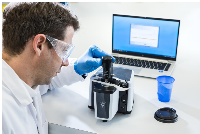
Figure 1. Agilent Cary 630 FTIR spectrometer coupled with a diamond attenuated total reflectance (ATR) module .
