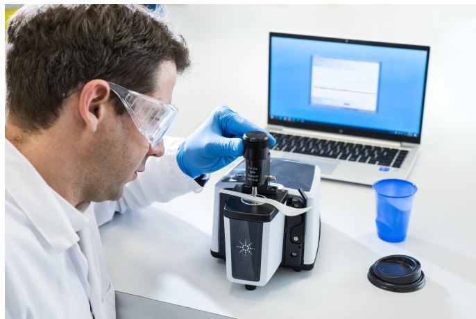
Figure 2. Agilent Cary 630 FTIR spectrometer coupled with a diamond attenuated total reflectance (ATR) module.
